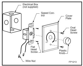
Fig. 10 Speed control mounting.
